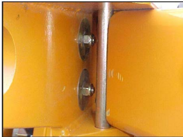
Fig. 5.01: Inner Tine Beam Shims
