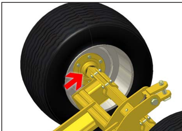
Fig. 5.10: Wheel Bearing Grease Points
