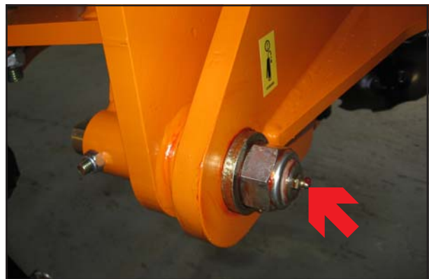
Fig. 5.09: Wing Pivot Grease Points
