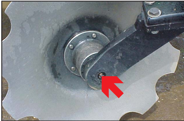
Fig. 5.04: Disc Hub Bearing Grease Point
