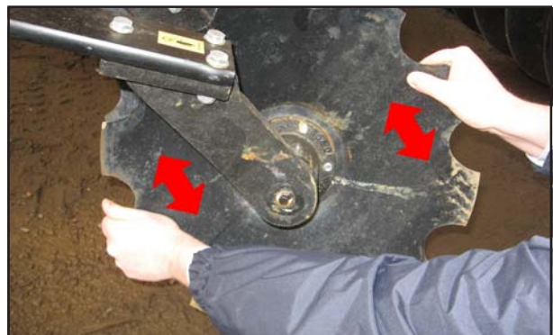
Fig. 5.01: Checking Disc Bearing Adjustment
