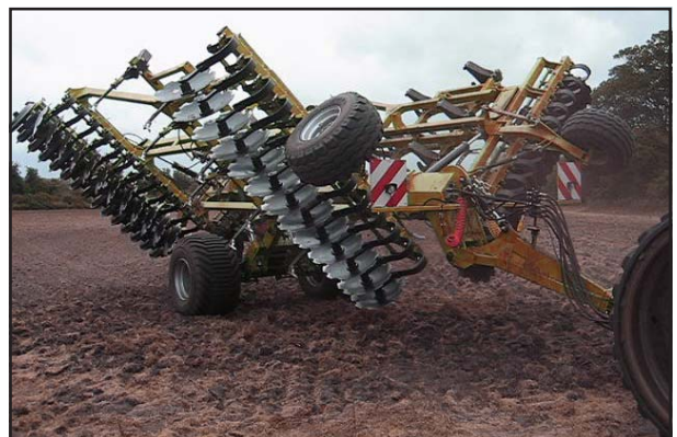
Fig. 2.04: Folding the SL700
