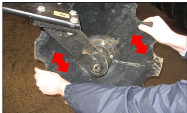
Fig. 5.01: Checking Disc Bearing Adjustment
