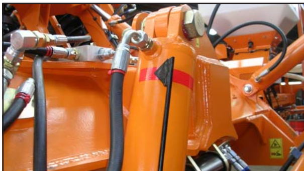
Fig. 2.02: Lift Cylinder Pointer and Marker
