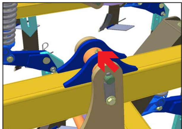
Fig. 5.06: Tine Frame Pivot Grease Points
