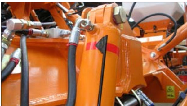
Fig. 2.02: Lift Cylinder Pointer and Marker
