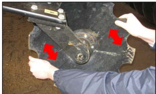
Fig. 5.01: Checking Disc Bearing Adjustment
