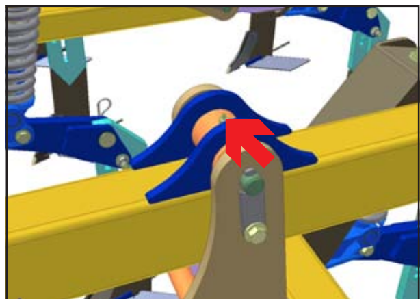
Fig. 5.06: Tine Frame Pivot Grease Points
