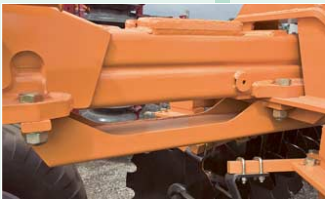
It is possible to convert a standard 300/330/380 to 'R' specification. Chassis bracket is required as part of the conversion.
