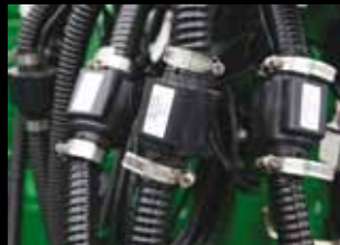
Blockage Monitors on each row notify the operator of any plugging.
