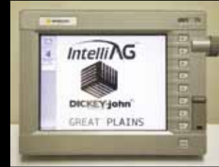
The ISOBUS compliant IntelliAG monitor manages seed rate, ground speed, shaft speed, bin levels and hose blockage.
