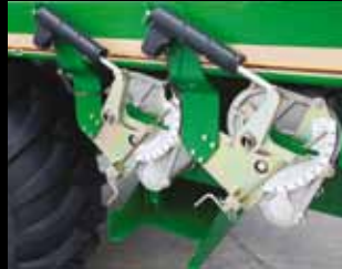
The step-less Infinite Ratio Gearbox allows you to set seed or fertiliser rates of each hopper independently.
