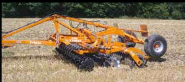
The trailing kit for the Mounted X-Press available for the Folding Wing model allows a tractor from 125hp to pull the 4m machine.
