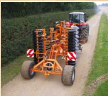
All models fold to a transport width of under 3 metres. Full European road lighting kit standard on all models
