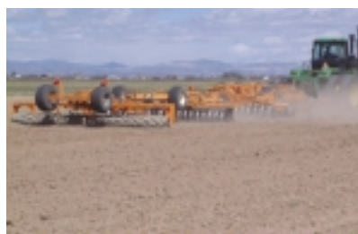
Solo and Aqueel press in a one pass system - Colorado, USA where consolidation of the soil surface and reduction of wind erosion is very important.
