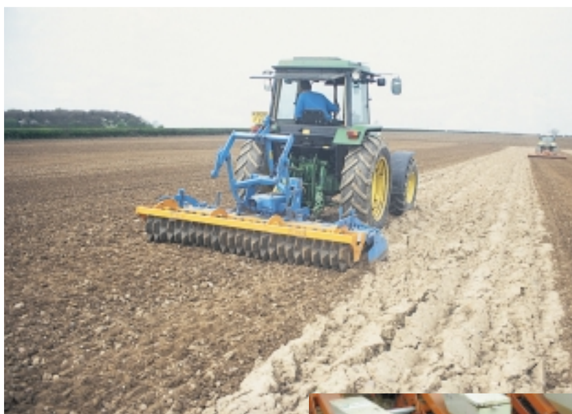
Nothing sticks to the Aqueel roller. Soil ridges retain moisture and prevent blow.
