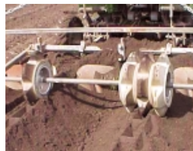
Single rimmed Aqueel on Potato ridges.
