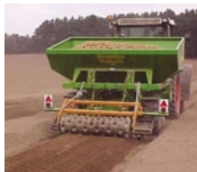
In conjunction with potato planters the Aqueel will firm the bed with the indentations being capable of retaining irrigated water until the crop is established.
