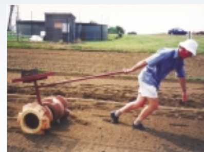
Dr. Tim Harrod pulling a prototype Aqueel press by hand and demonstrating that the Aqueel can be human powered for use in developing countries
