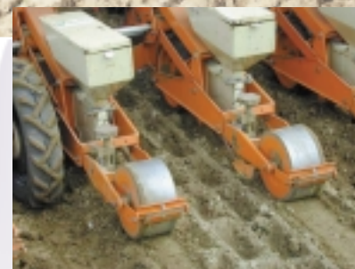
Nothing sticks to the Aqueel roller. Soil ridges retain moisture and prevent blow.
