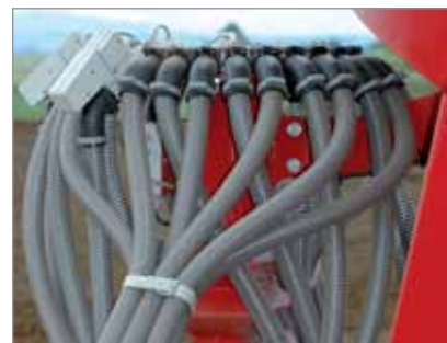
The distribution head is located outside the hopper for ease of access
