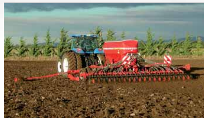
The leading discs create a good tilth
