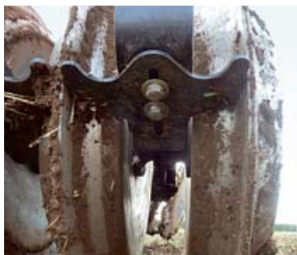
One-piece scrapers are now proven and did a good job on the test field's wet heath land.
