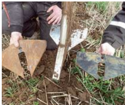
There are three SLD wing options: 300mm wide, 250mm standard and similar width Lo-Lift wings. The Lo-Lift wings work at a shallower angle for less surface disturbance.
