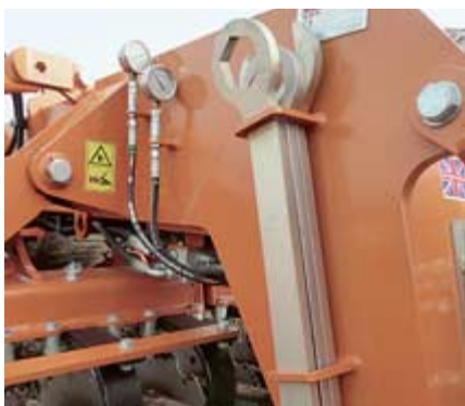
SLD leg trip pressure can be set up to 90 bar, giving a trip force of nearly 1,500kg. Onboard DD spanners are part of the Simba package.
