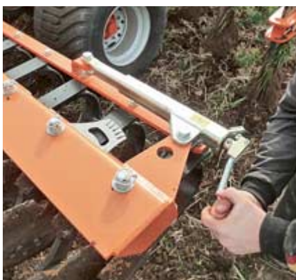
The disc angle can be set up to 25° using the winder. Simba suggests starting at a flat angle and then working steeper when setting up.
