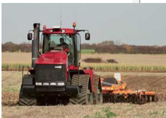
Designed for plenty of up-front muscle, the 6m SLD needs a minimum of 400hp. Here it's towed by a 543hp Quadtrac.
