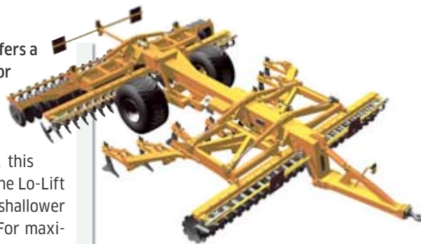
The final version will have nine instead of ten tines and a single ram on the drawbar.
