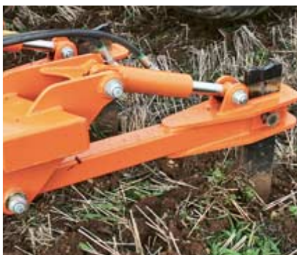
Each of the seven (4.6m) and nine (6.0m) tines on the SLD has hydraulic auto-reset.
