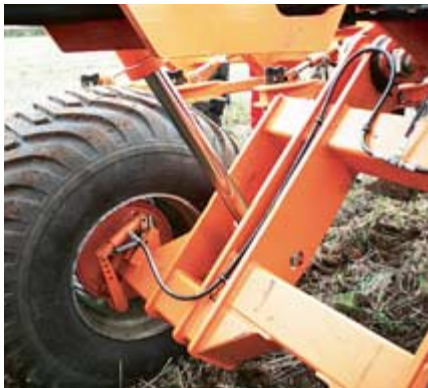
Hydraulic brakes are part of the standard spec, and there's also a pneumatic option. Production machines will use a beam axle.
