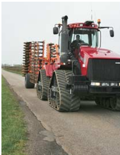
On-road transport width is 3m. Overall height of the folded 6.0m model will be 3.975m.
