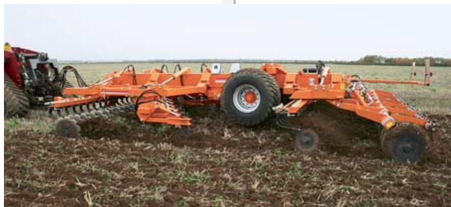
This 6m SLD prototype is based on a Solo 600 frame and was working in the UK all last season. Cultivation layout is discs, tines, discs with a rear packer, with the option to pull a second press.
